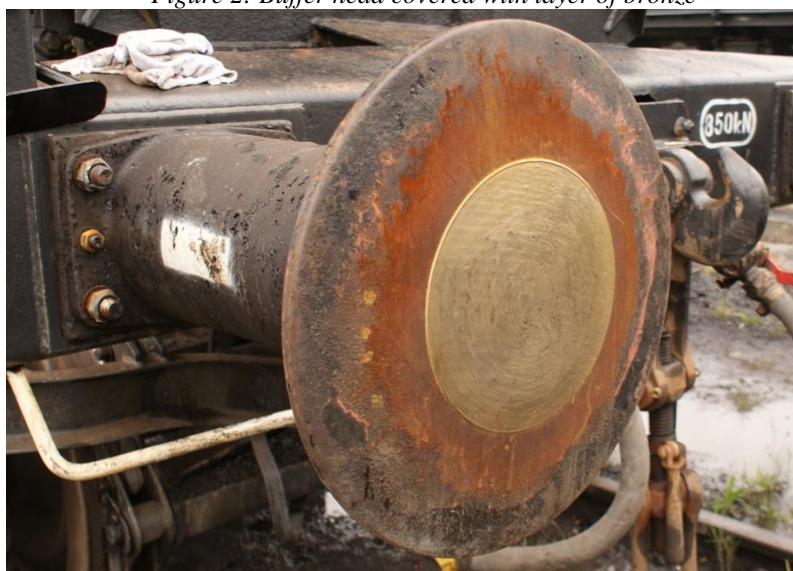
Figure 2: Buffer head covered with layer of bronze
