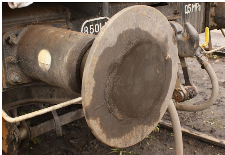
Figure 1: Buffer head covered with grease
